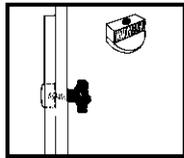
Slide Guides make angle and height adjustments on Best easels smooth. These circular graphite impregnated plastic inserts are used wherever there is a slot in the wood of the
