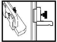
The Elevator Bolt Locking System is used on top trays. The 2 metal plates and round plastic guide keep the parts parallel which allows for smoothness
