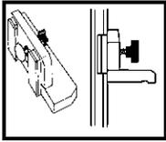
The Elevator Bolt Locking System is used on top trays on Best easels. The 2 metal plates and round plastic guide keep the parts parallel which allows for smoothness and ease when the tray is moved
