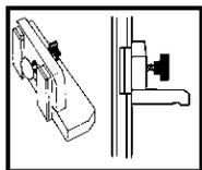
The Elevator Bolt Locking System is used on top trays on Best easels. The 2 metal plates and round plastic guide keep the parts
