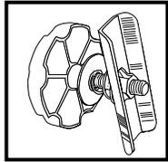
Height & tray adjustments unlock easily, yet lock into place & stay locked because of the **Wedge-lok System**. The metal plate features wedge-cut edges that conform
