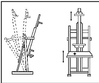
To change position of the painting trays: Loosen or disassemble the **Wedge-Lok System** slide or place in desired position and reassemble or tighten.
