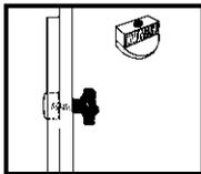
**Slide Guides** make angle and height adjustments on Best easels smooth. These circular graphite impregnated plastic inserts are used wherever there is a slot in the wood of the easel. This part allows for smooth movement and protects the hardwood from the metal bolt.
