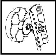
Height & tray adjustments unlock easily, yet lock into place & stay locked because of the **Wedge-Lok System**. The metal plate features wedge-cut edges that conform to the wedge-cut sections of the hardwood. When the knob is tightened, the inward tension pulls the metal plate snugly against the wood for a solid lock.
