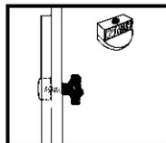
**Slide Guides** make angle and height adjustments on Best easels smooth. These circular graphite impregnated plastic inserts are used wherever there is a slot in the wood of the easel. This
